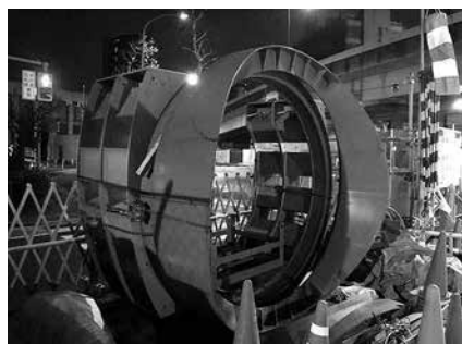
写真-1 刃口式推進機全景 (推進機外径2,600mm)
